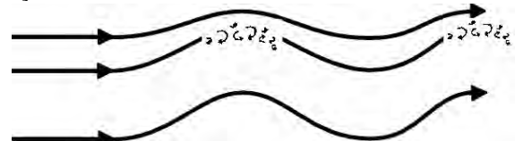
Figure 6c Turbulence in wave-crests caused by augmenting shear which is due to declining amplitudes with increasing altitude [Source: Wallington 1 p.230]
