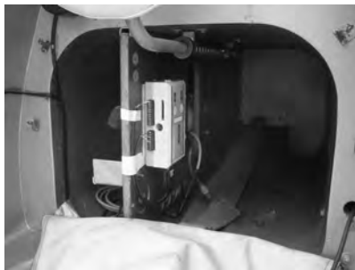
Figure 4 The GPS-data-logger MPL-3440 mounted in a SZD 24-4A Foka 4
