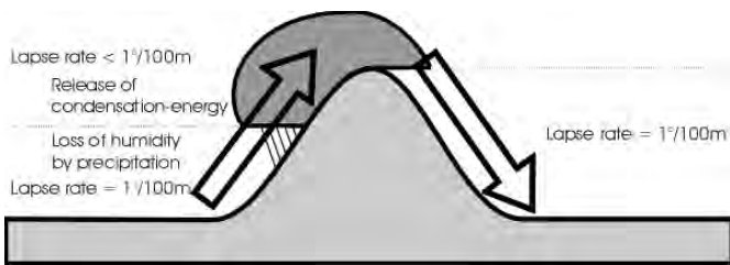
Figure 13 Classic thermodynamical foehn-principle or “Swiss-foehn” after Hann 6 quoted according to Steinacker 7 , p.4]
