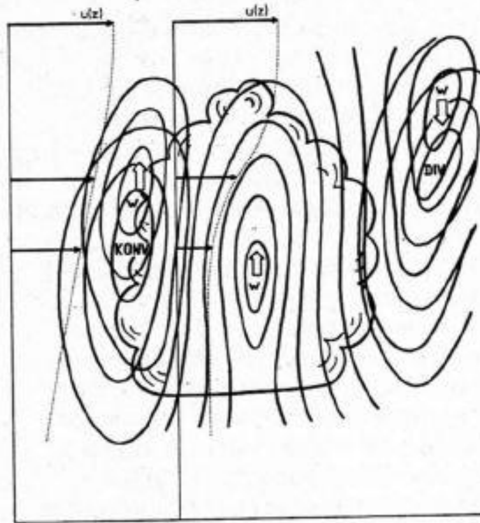
Figure 4 Model of thermal wave surrounding a cumulus cloud. Vertical velocities, w , and convergence and divergence pattern are indicated. The vertical profiles of the horizontal wind inside and outside the cloud are also shown.
